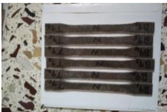
Fig.5: Hybrid 9% flyash composite
