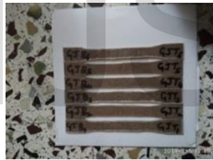
Fig.2: Jute & E-glass composite
