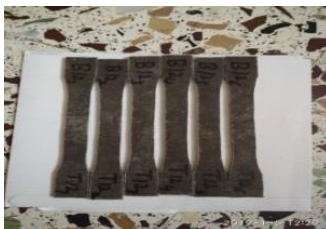
Fig.6: Hybrid 12% flyash composite
