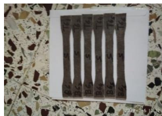
Fig.4: Hybrid 6% flyash composite
